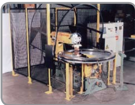
Fleximan With Programmable Rotary Table For The Production Of Fan Guards
