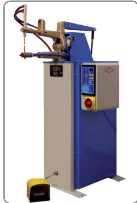
AS15BCT Air Operated Spot Welder
