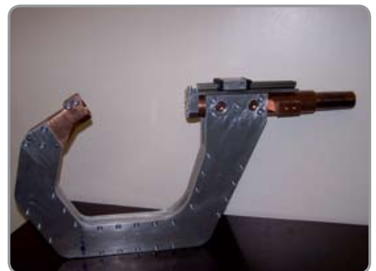
Modular robot gun arms with linear slides made from both high strength aluminium and CuCrZr.
