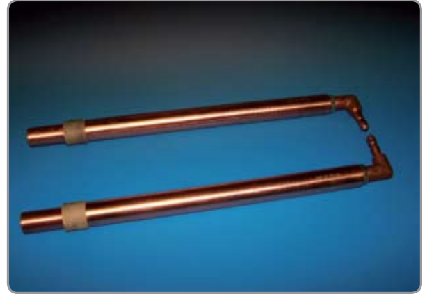
CuCrZr manual welding gun arms with cast holders
