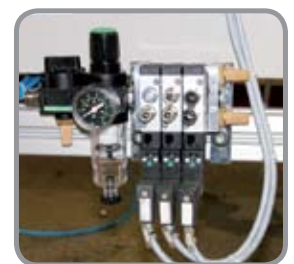
Pneumatic unit with filter and self-governing relay.
