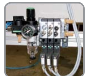
Pneumatic unit with filter and self-governing relay.
